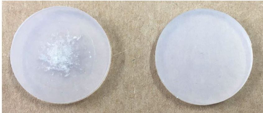
Fig.: The worn septum (left) must be replaced.
